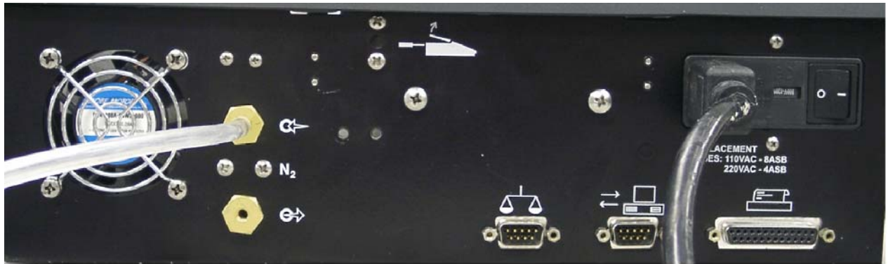
Dry Air Inlet with Tygon 2075 tubing connected
