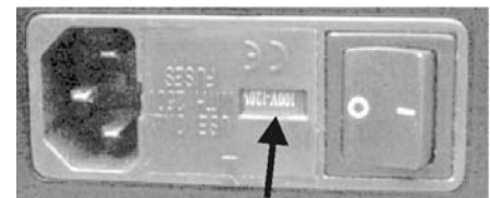
Voltage setting appears in window (110V-120V or 220V-240V)
