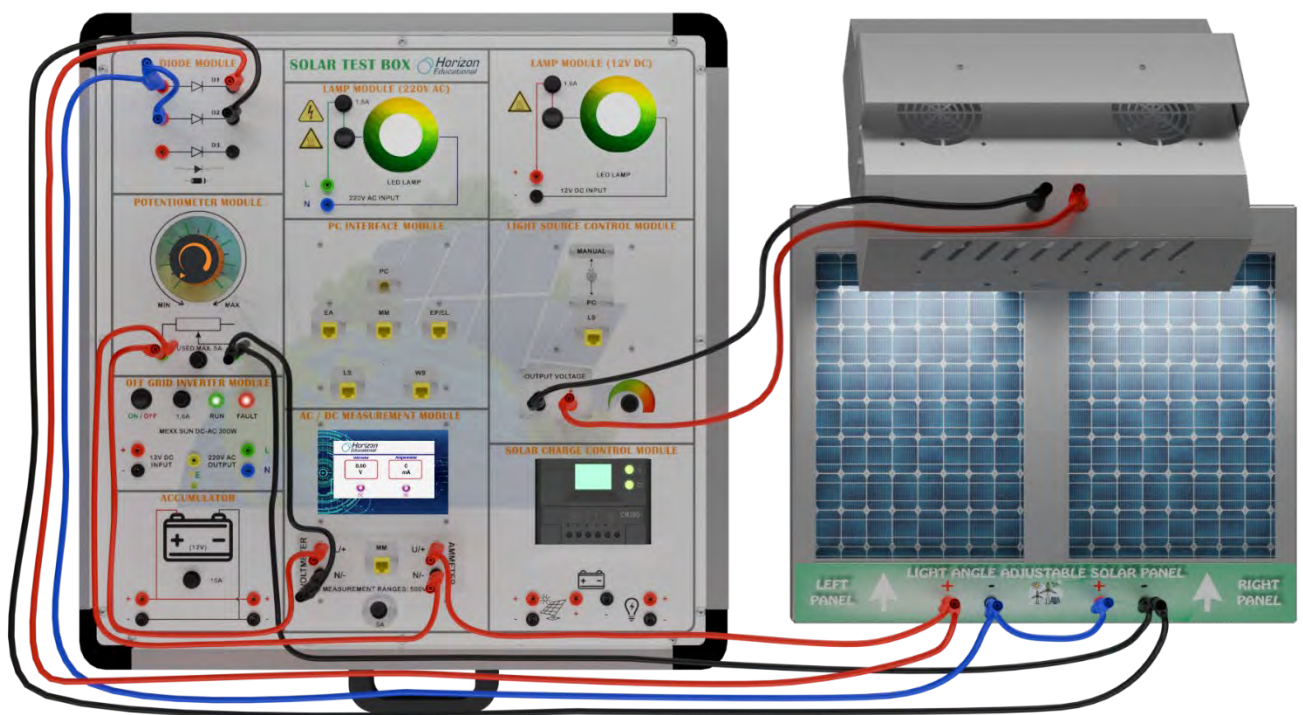
Figure-32. Installation Image of Examination of Effect of Bypass Diode in Photovoltaic Panels
