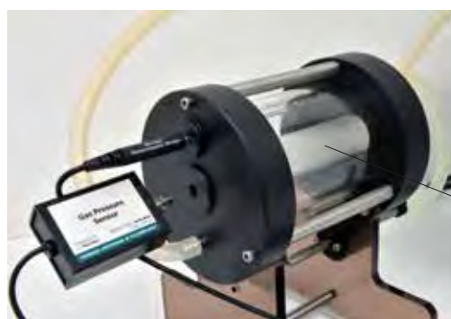
CH-0010-00 Cylindrical Water Jacket ■ Material Type: Glass and Hard PLastic ■ Diameter: 12 cm
