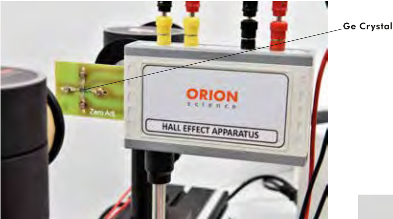
EE-0160-00 Hall Effect Apparatus Controlled voltage is applied to germanium crystal. Hall voltage is measured by multimeter.
