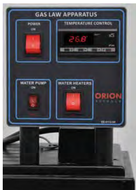
EE-0110-00 Heater and Pump Control Unit ■ Temperature Control ■ Maximum Temperature 70°C
