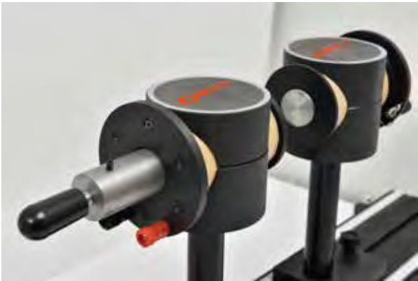
EE-0161-00 Solenoids The magnetic field on the germanium semiconductor is changed by the current supplied to the solenoids.
