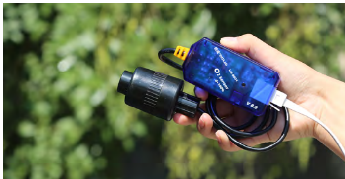
Measuring O 2 content in forest with O 2 sensor
