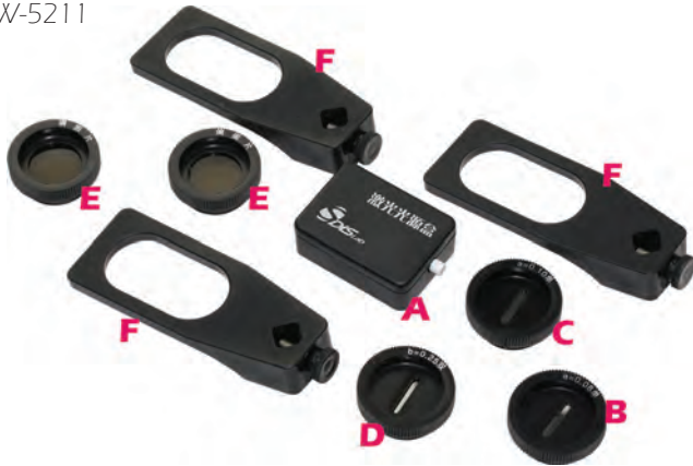
0.25mm double slit on the specialized bracket
