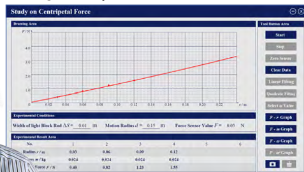
Experiment fitting curve F-r on the centripetal force and radius
