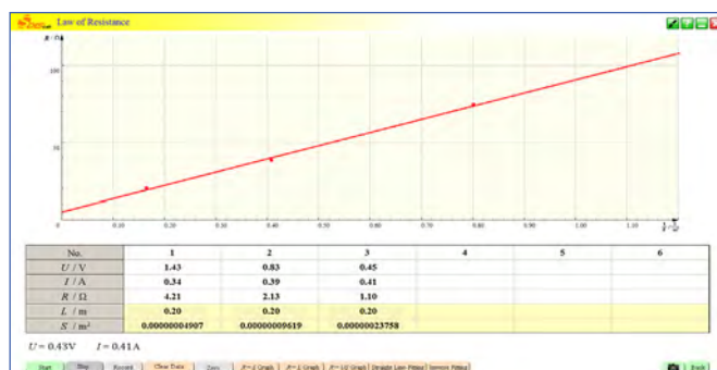
Relationship between resistance of metal wire and the reciprocal of its cross section
