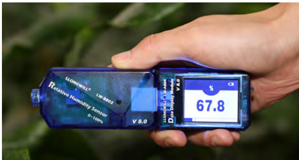
Relative humidity sensor connected to Sensor Data Display Module
