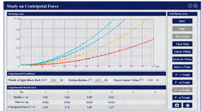
Curve of relationship between centripetal force F and angular velocity \omega
