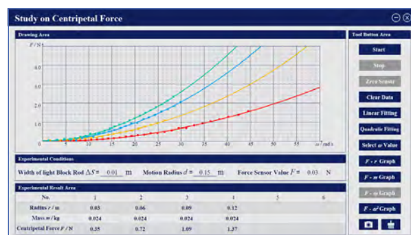
Experiment results of the relationship between the centripetal force F and angular velocity \omega
