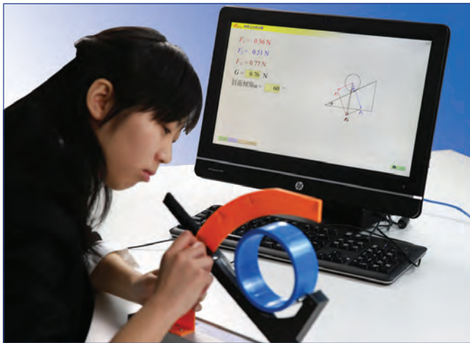
The readings of two force sensors at 30^\circ angle
