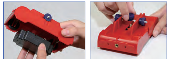
Assemble the scanner into the cart
