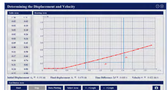
The experiment results of measuring the displacement and velocity by using our digital photoelectric track
