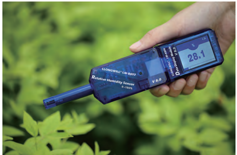
Measuring the ambient relative humidity using relative humidity sensor and sensor data display module
