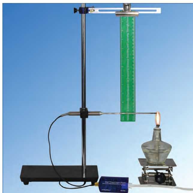
Measure the temperature of different parts of alcohol lamp flame, results as below
