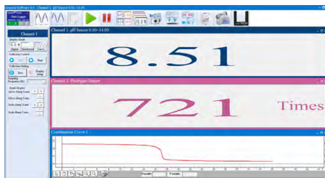
The results of Acid-base Neutralization Titration by using pH sensor
