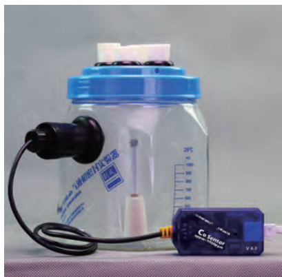
Experiment of CO content generated during cigarette combustion measured by using CO sensor
