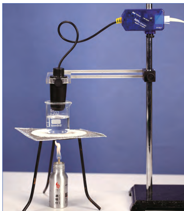
Detection of NH 4 + with NH 3 sensor
