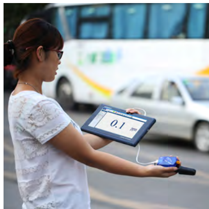
Experiment of testing of NO 2 content in vehicle exhaust with NO 2 sensor and digital display module
