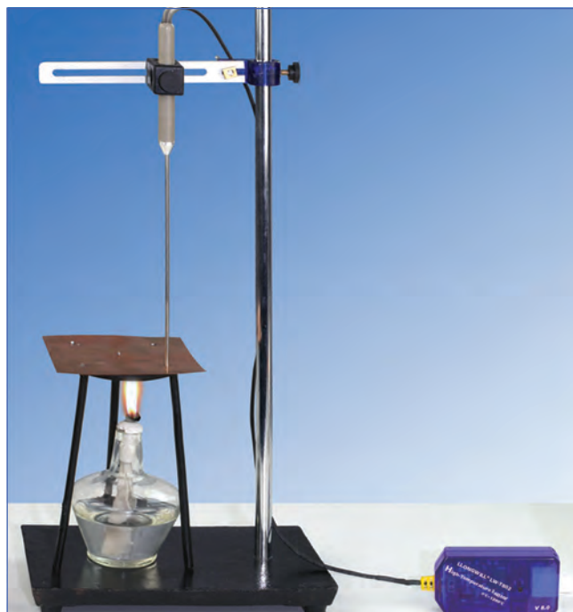
Measure and compare melting temperatures of soldering tin, tin and lead
