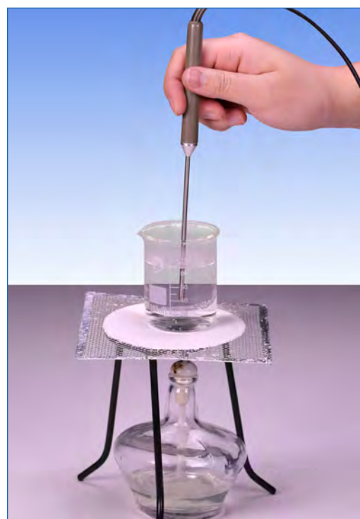
Fig. 2-25 Experimental Installation for The Study of Boiling Water
