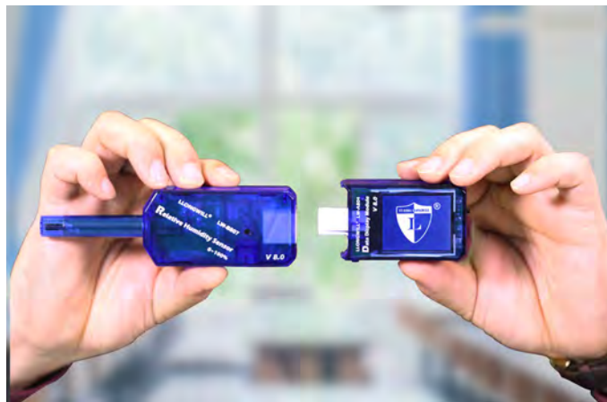
Fig. 2-1 Connecting the data display module with the sensors
