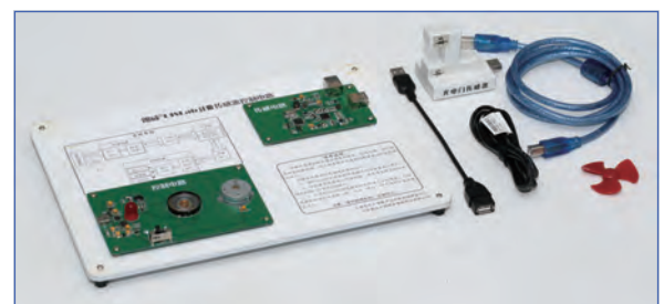
Counting sensor control circuit
