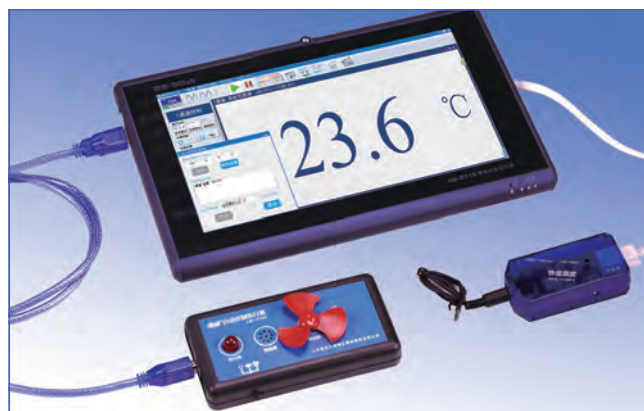
An automatic control system composed of Pad terminal, actuator and fast response temperature sensor
