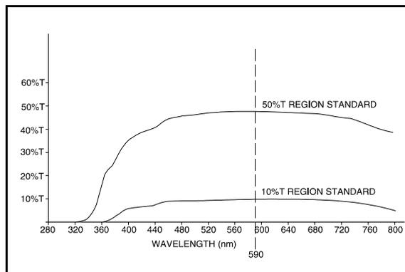
Figure 3. Transmittance/Wavelength Profile of Photometric Performance Standards
