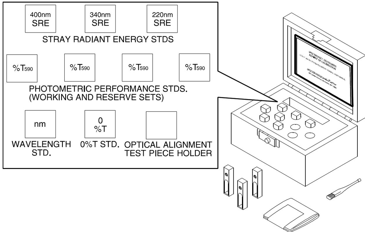
All standards have the same external dimensions as a 10mm-pathlength square cuvette, so they will fit in practically any spectrophotometer that accepts such cuvettes. Adapters that permit the standards to be used in Thermo Spectronic test-tube-holder sample compartments are described under Accessories.
