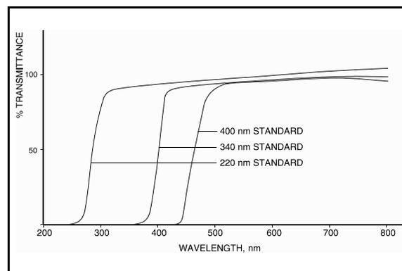
Figure 2. Transmittance/Wavelength Profile of Stray Radiant Energy Standards
