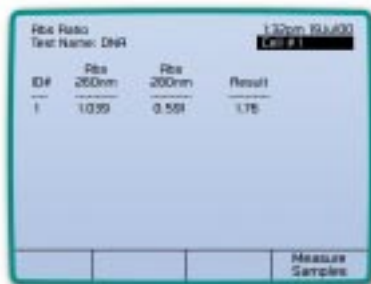
Results of DNA purity measurement showing test name, absorbance values and out-of-range indication
