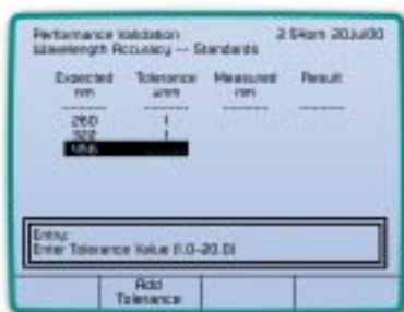
Screen used to enter desired wavelength accuracy tolerance
